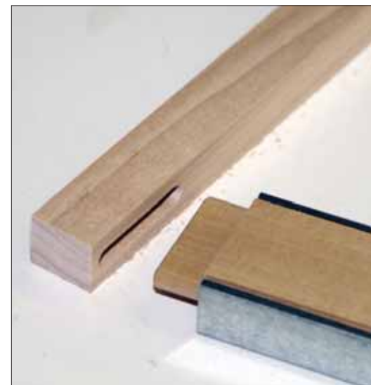
(top) Poplar boards going through a table saw to make blank screen frame styles and rails. (middle) Dave Lowell operates the twin-table round-end tenoner. (bottom) The slot mortiser in action. (right) Completed style and rail with rounded tenon ready to be glued and assembled. (Joe Funk photos)
